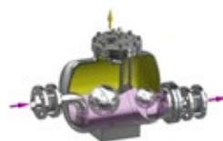
**6.** As the motive steam valve closes and the vent valve opens, equalizing the body pressure with the upstream pressure allowing condensate to flow once again into the APST. The cycle then repeats itself and with enough differential pressure, the system resumes as a steam trap, or otherwise, as a pump.
