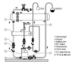
Drainage of a single unit under vacuum (max. 0,2bar abs).
