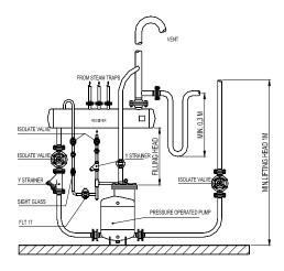
Removal of condensate under pressure with POP pump and steam trap combination. When the steam pressure is sufficient to overcome back pressure the trap operates.
