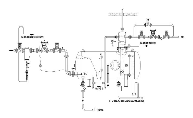
Atmospheric deaerator provides an economic system to preheat boiler feed water and drive off dissolved gasses.
