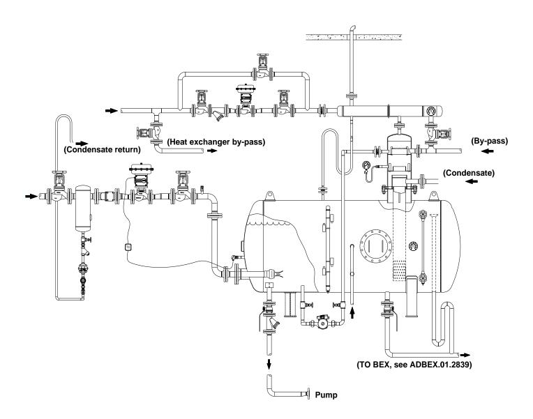
Atmospheric deaerator including Adcatherm-STS series complete stainless steel heat exchanger. Make up water crossing the heat exchanger will condense the flash steam, preventing energy waste and better performance of the whole system.
