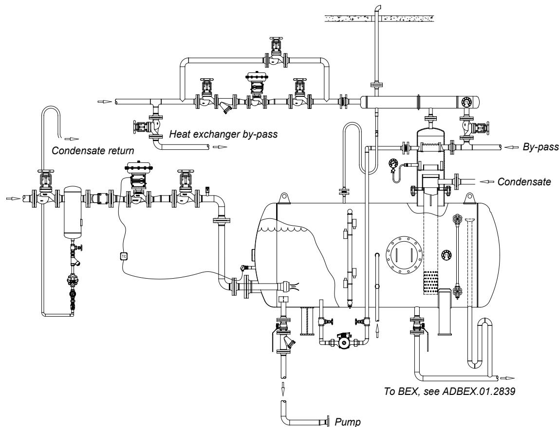
Atmospheric deaerator including ADCATherm STS series complete stainless steel heat exchanger. Make-up water crossing the heat exchanger will condense the flash steam, preventing energy waste and providing better performance for the whole system.
