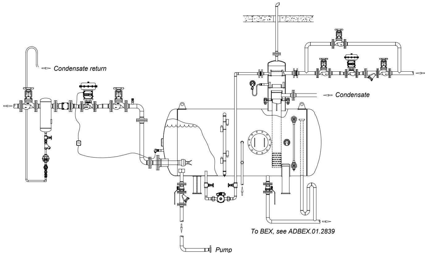
Atmospheric deaerator provides an economic system to preheat boiler feed water and remove dissolved gases.
