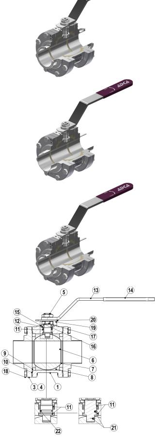
$<sup>^{\</sup>star\star}$  Loose flange. Allows a 360° rotation of the valve when using tube weld connections.
