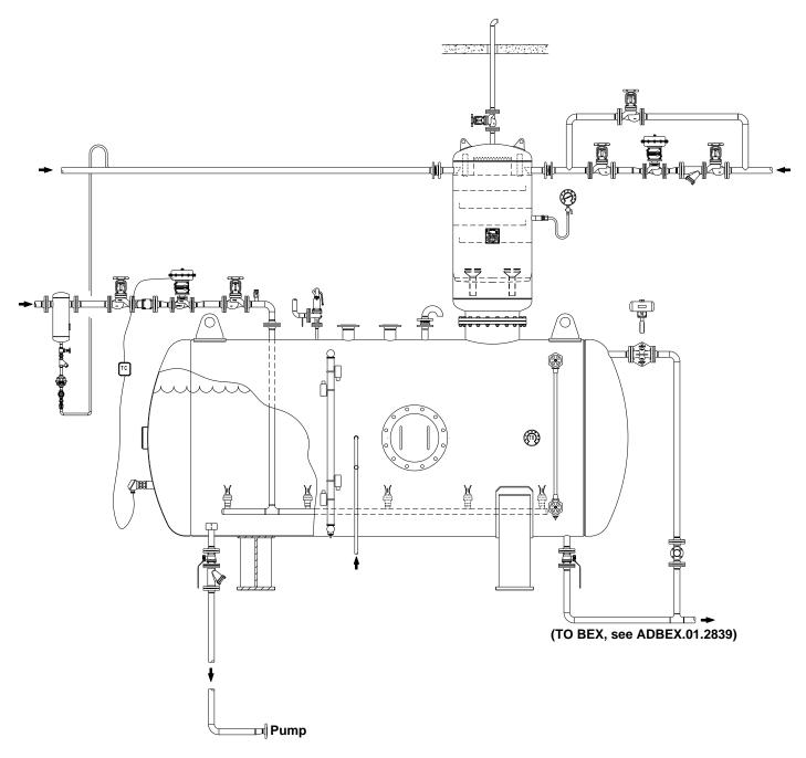
If a high percentage of hot condensate is recovered, the direct steam injection in the deaerator tower is usually unnecessary, as the heating steam supplied trough the steam injection system is, in most cases, enough.
