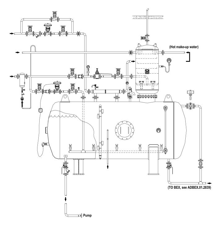
Thermal deaerator with low pressure steam to water Adcatherm-STS complete stainless steel heat exchanger, providing make up water heating.
