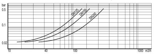
Pressure drop, horizontal flow, standard spring (water - 20°)
