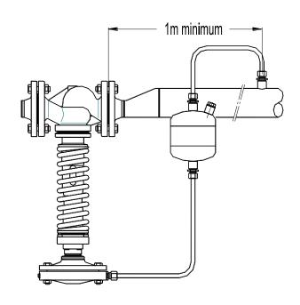
By-pass: if overpressure can not be accepted, the use of a by-pass is not recommended. In alternative, for critical processes, two pressure reducing stations should be installed in parallel.
